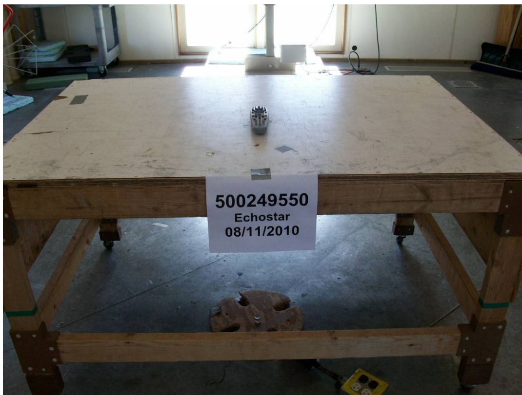
Test Setup – Radiated Emissions (Rear View)
