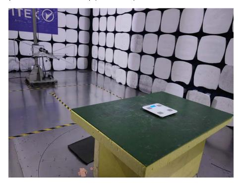
Spurious Emission Test Setup (Above 1GHz)
