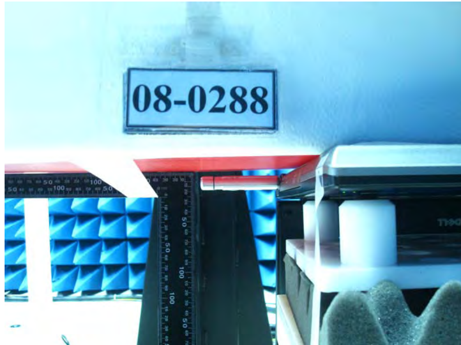
Figure 19. Body SAR Test Setup (Flat Section) _ EUT Horizontal Up
