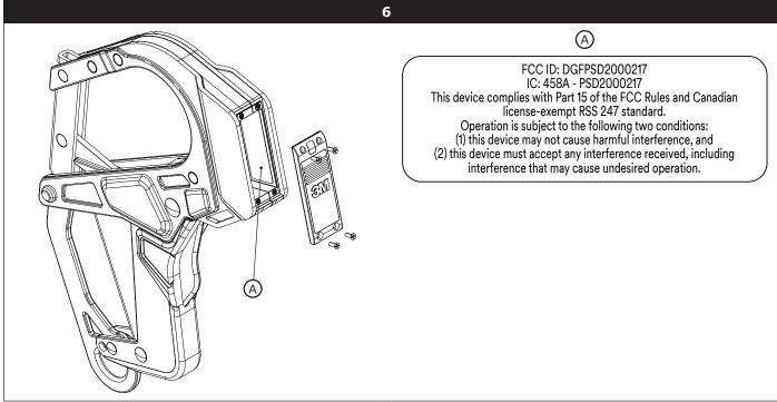
$\ensuremath{\overline{\bigvee}}$  Before using this equipment, record the product identification information from the ID label in the `Inspection and Maintenance Log' at the back of this manual.
