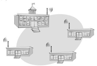
In this configuration, the wireless bridges make all four wired LANs appear to be connected by the same Ethernet cable. Using wireless bridges in this manner provides a cost-effective way to wirelessly link multiple wired LAN networks by eliminating the need to install cables between buildings.
