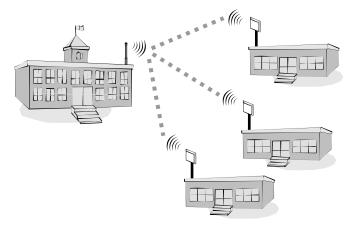
In this example, the first building's bridge is using an omnidirectional antenna while the other three buildings have bridges using directional antennas. In this case, the three bridges with directional antennas can communicate only with the bridge using the omnidirection antenna; they cannot communicate directly with each other. The bridge using the omnidirectional antenna can communicate with the other three bridges.
