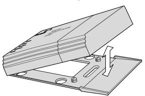
**3** To mount the bridge, install the mounting plate where desired using the mounting hardware provided (see "Physical Dimensions" on page 6 for the physical dimensions of the mounting plate).
