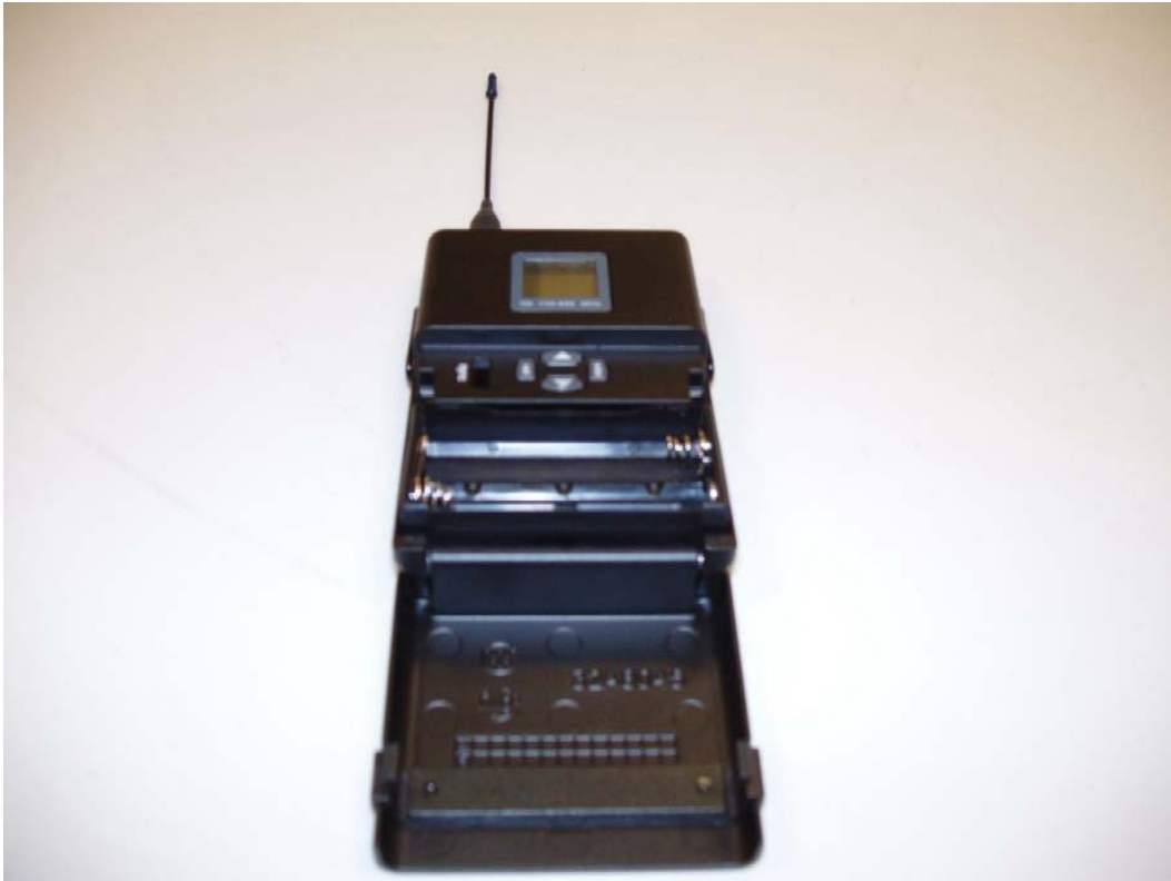
Shure UR1A Front View – Battery Door Open
