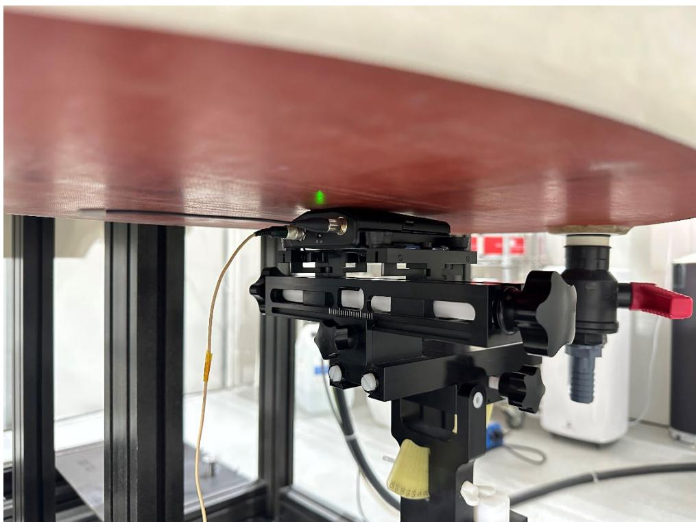
Description: Body Back Position with 0mm gap for TQG audio connector
