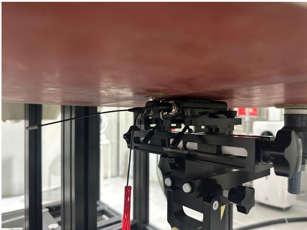
Description: Body Left Position with 0mm gap for TQG audio connector
