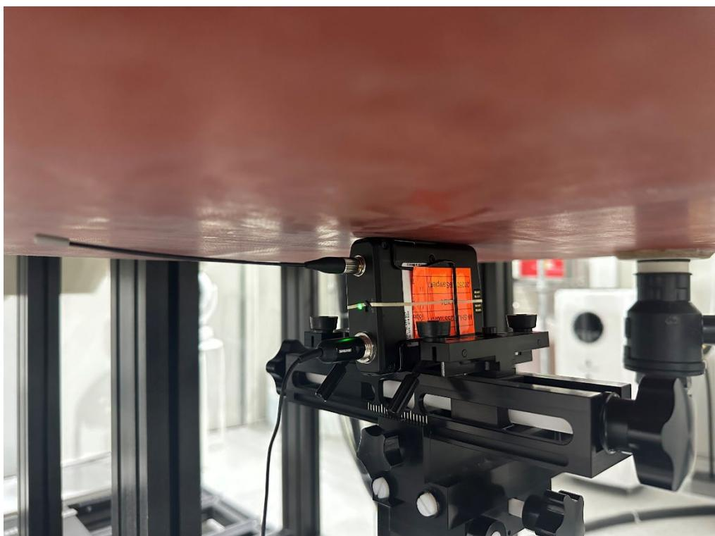
Description: Body Right Position with 0mm gap for TQG audio connector
