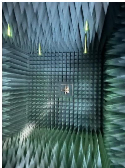
Figure 4 – Diagram of Shure antenna chamber. Designed per ETSI EN 300 422-1, section D-1
