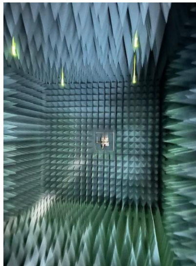
Figure 5 – Photo of Shure Antenna Test Chamber.
