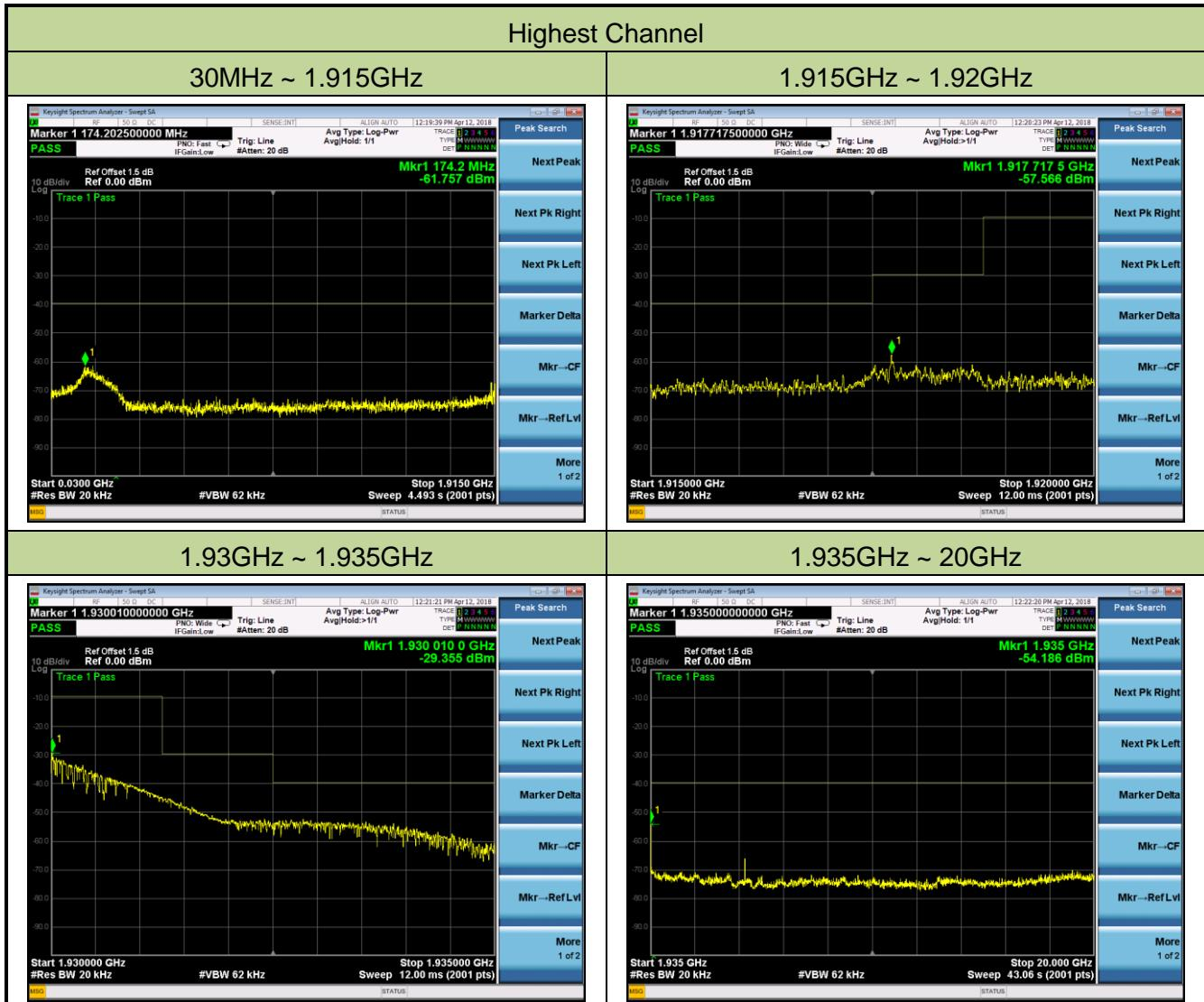
Note: The BS spurious out-of-band transmission level is below the indicated limit.
