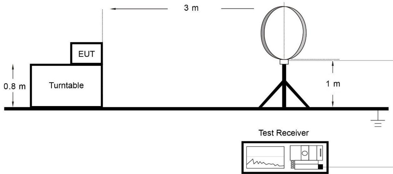
Below 1GHz Test Setup:
