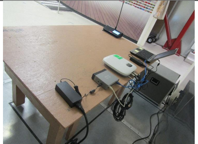
AC Conducted Emissions – Side View
