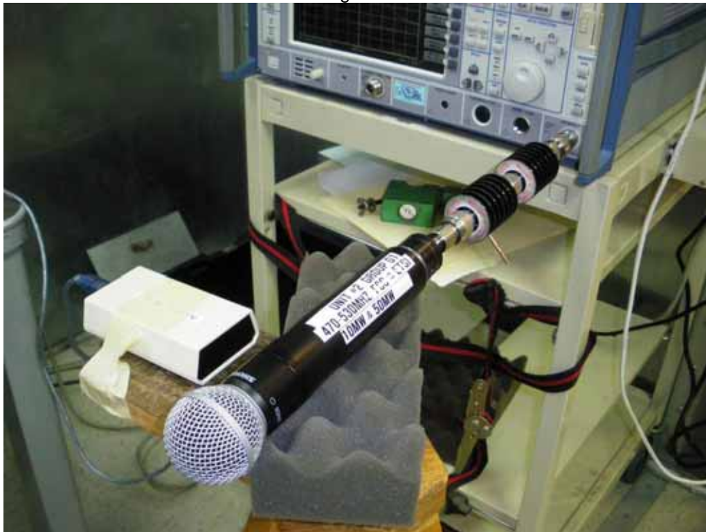
Test Set-up for RF Power Output Test
