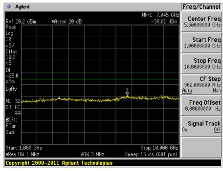
Note: The limit line in above plots is based on IC limit; however, FCC limit line is -13 dBm. Plots comply with both FCC and IC requirements.
