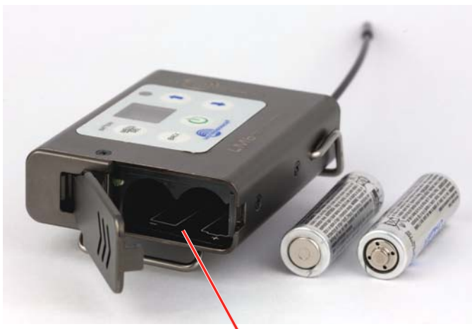
Battery polarity is marked inside the compartment
