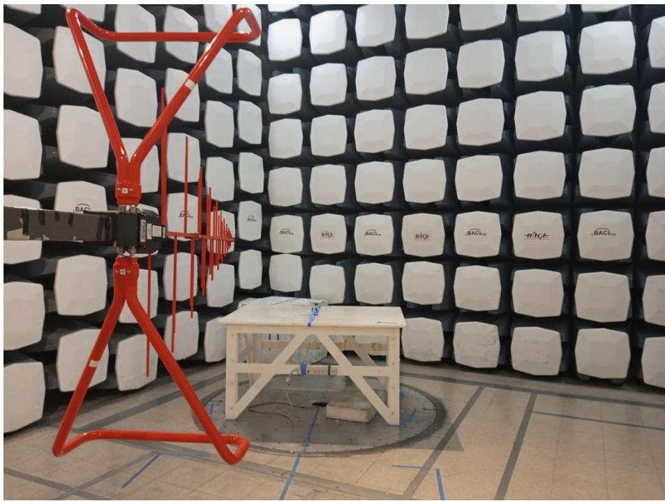
**1.4 Radiated Spurious Emissions: Below 1 GHz, Rear View at 3 meters distance (Vasona)**
