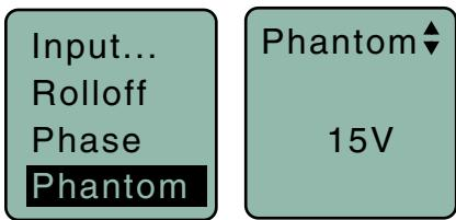
The transmitter input jack can provide phantom power for the attached microphone if needed, with voltages at 5, 15 or 48. Phantom power will consume a slight amount of battery power, so it can also be turned off.
