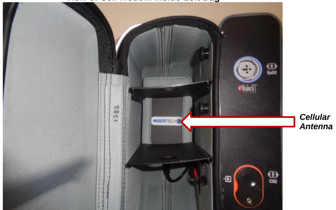
View of Cell Modem Inside Left Bag
