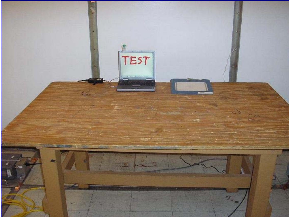
Photograph 2. Conducted Emissions Test Setup with Power Supply Model: LF91000D-41
