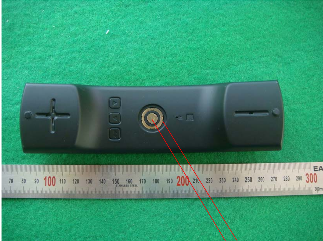
<Photograph 6: Battery charging point>
