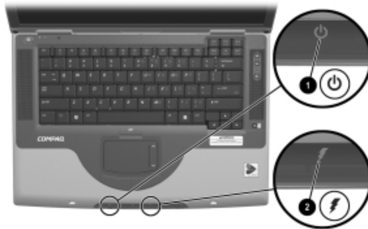
Identifying the battery and power/standby lights
