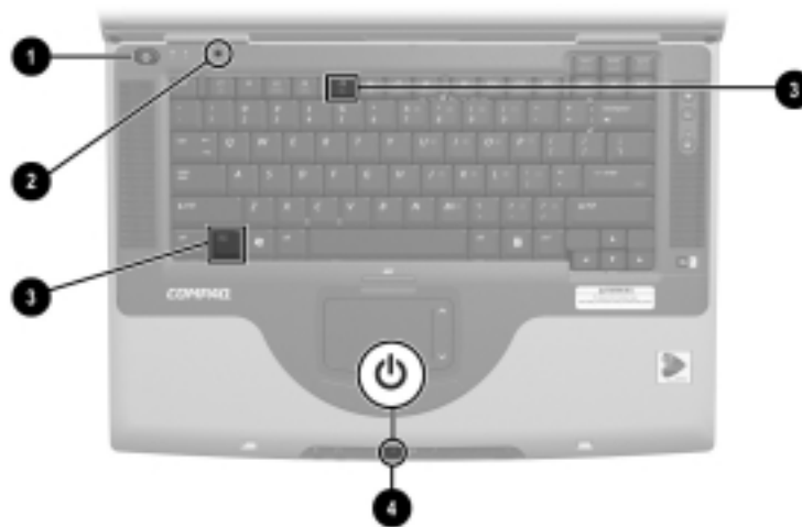
Identifying Standby, Hibernation, shutdown, and display controls and indicators
