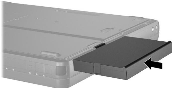
To remove a MultiBay battery pack, turn the notebook upside down. Then slide and hold the MultiBay release latch ① as you pull the battery pack ② from the MultiBay.
