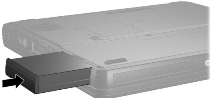
To remove a battery pack, turn the notebook upside down. Then slide and hold the battery release latch **1** as you pull the battery pack **2** from the battery bay.
