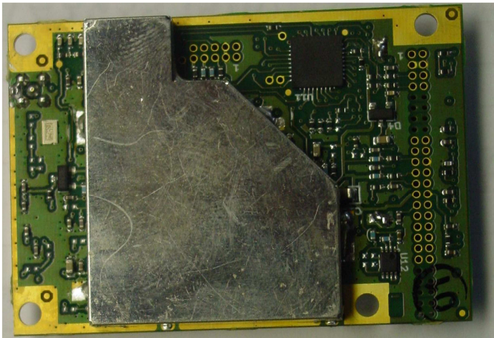
LRM 450MHz 79543TRX BOTTOM with Shielding
