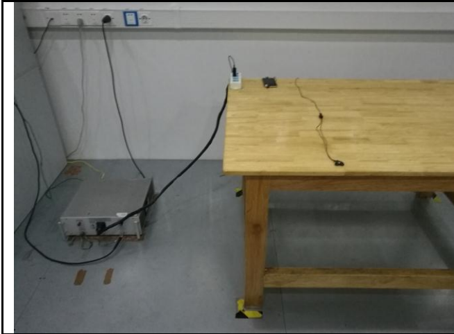
Conducted Emissions Test Setup Front View
