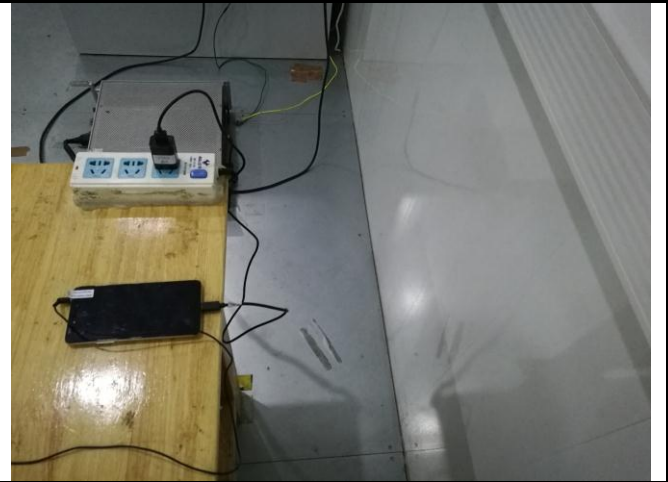
Conducted Emissions Test Setup Side View
