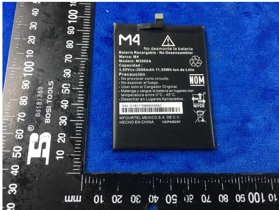
Battery - Front View
