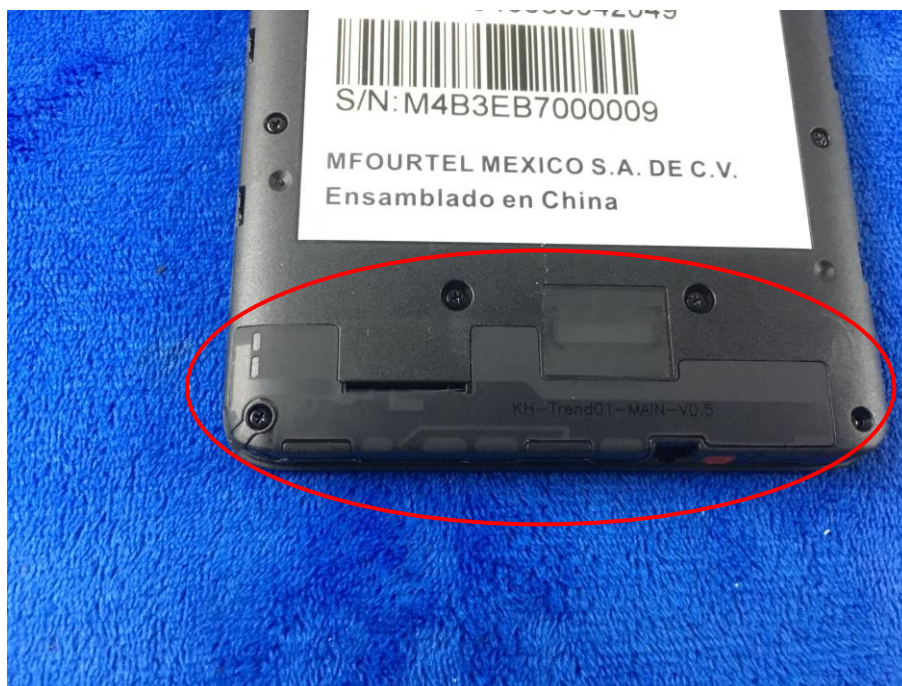
GSM/PCS/UMTS-FDD/LTE Antenna View
