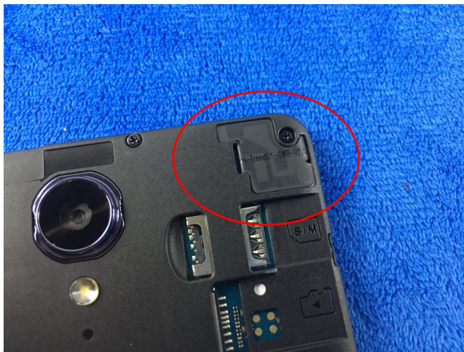
WIFI/BT/BLE/GPS - Antenna View
