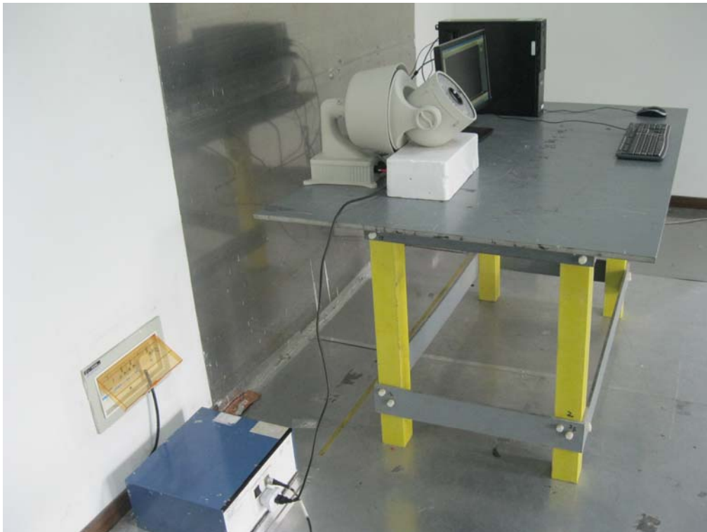
Conducted Emissions Test Setup - Side View
