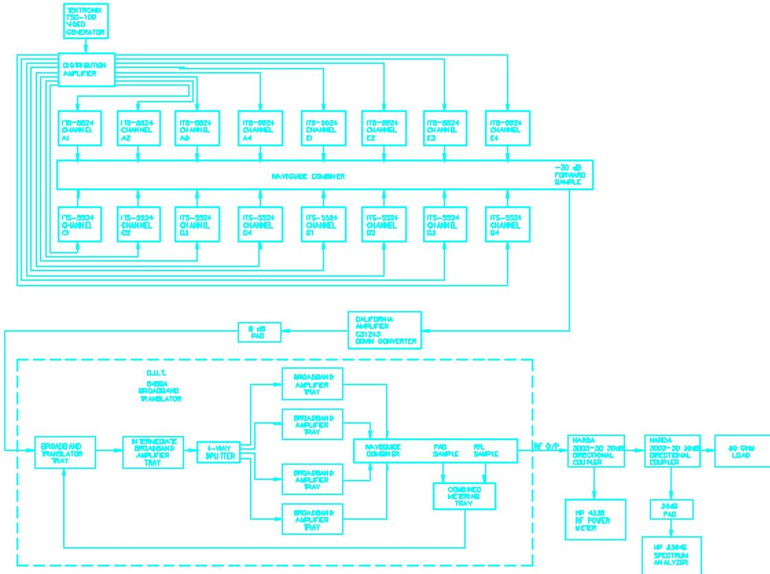
Before testing the 6459A multi-channel translator, the ITS-5724 transmitters (FCC ID# CJ79SITS-7022) used to generate the multi-channel input signal to the translator were tested and observed to meet specifications. Then, the translator was tested and observed, as illustrated in the following sections, to reliably reproduce the transmitted signals in accordance with the rules set forth in the Rules and Regulations.
