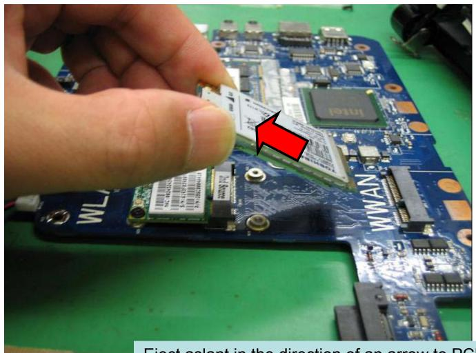
Eject aslant in the direction of an arrow to PCB side.
