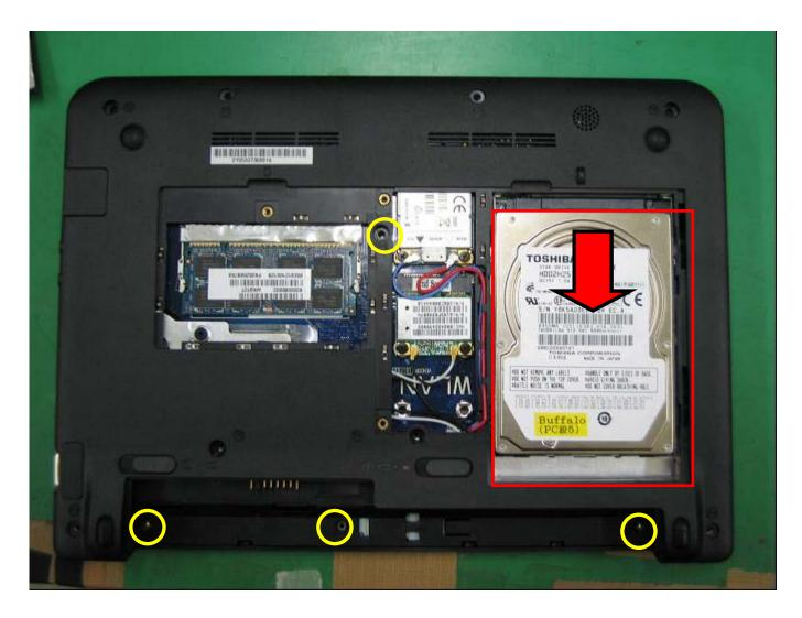
HDD and a screw are removed.
