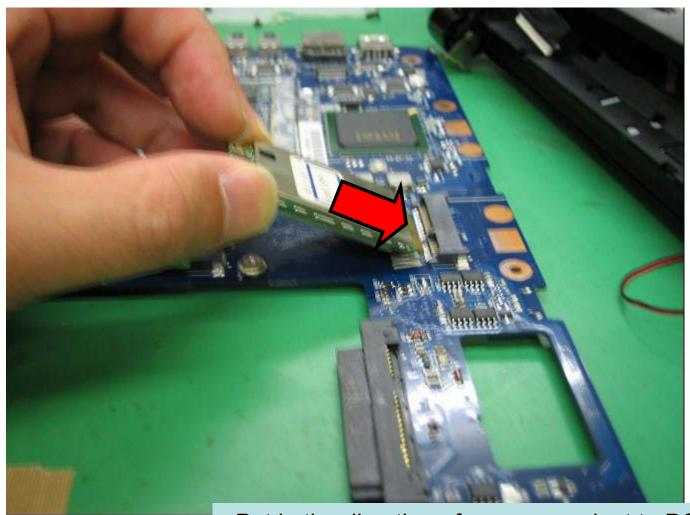
Put in the direction of an arrow aslant to PCB side.
