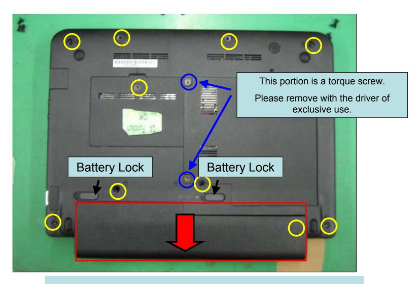
Battery and a screw are removed.
