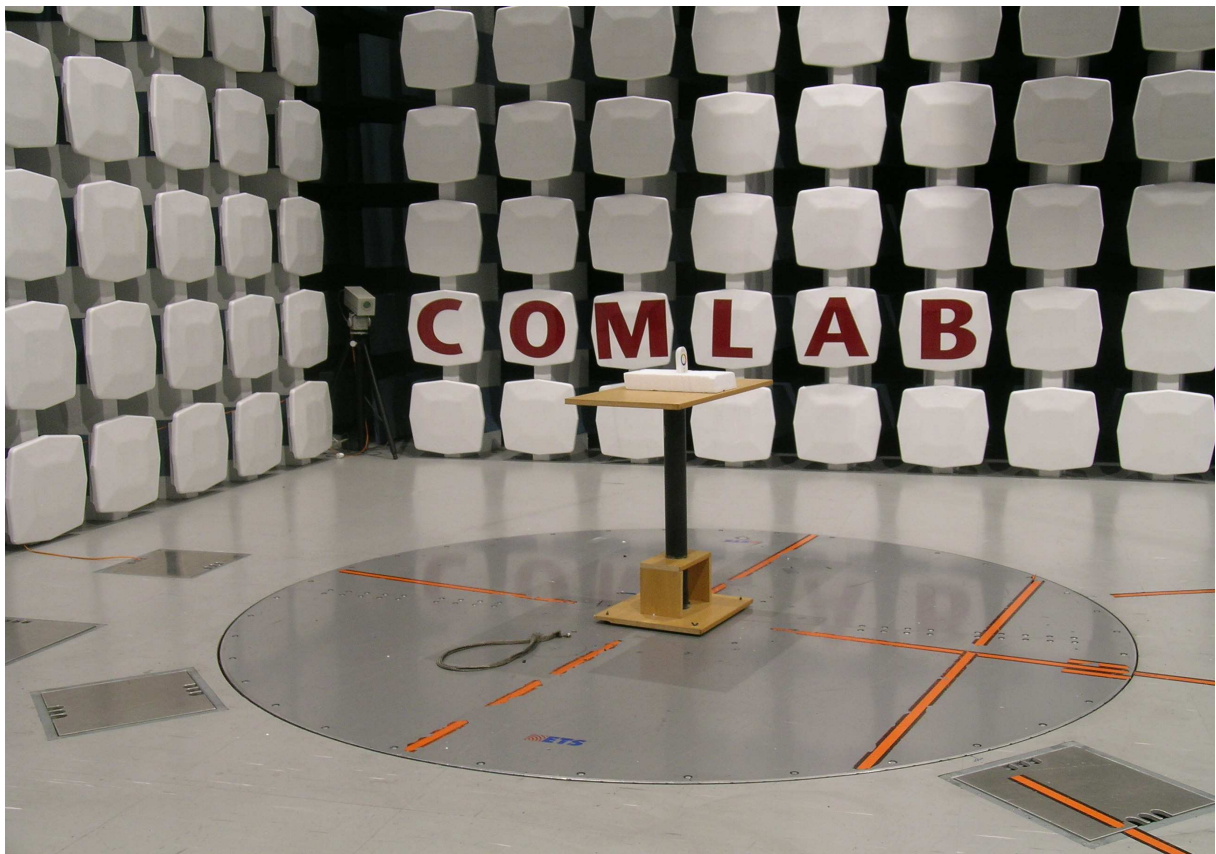
Radiated Emissions Test above 30 MHz @10m
