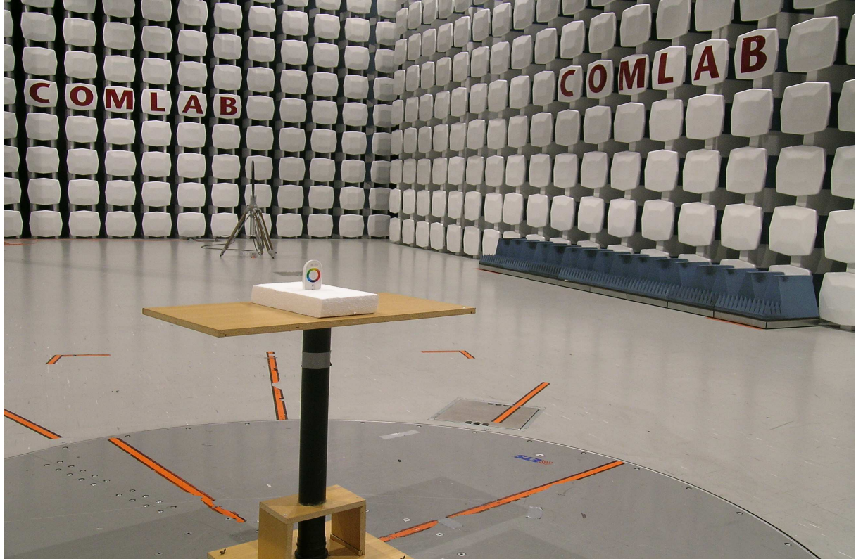
Radiated Emissions Test below 30 MHz @10m
