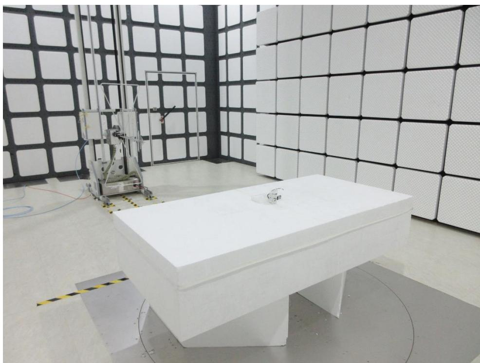
**Test Mode: Mode 1****Description: Radiated Emission Test Setup for above 1GHz**
