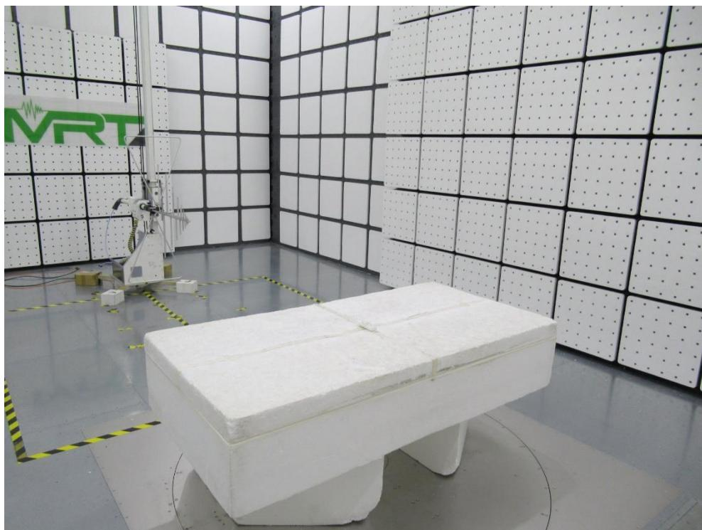
**Test Mode: Mode 1****Description: Radiated Emission Test Setup for above 1GHz**
