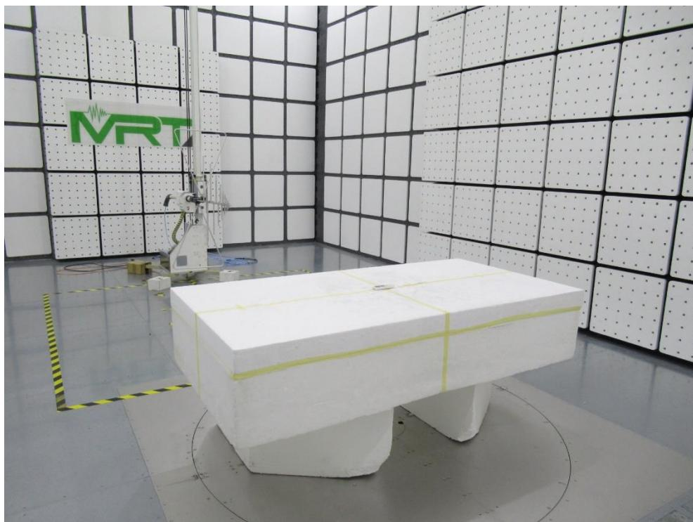
**Description: Radiated Emission Test Setup for above 1GHz**
