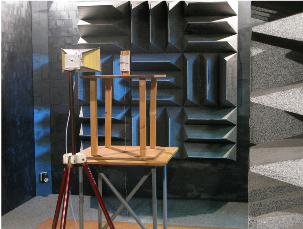
Photograph 3: Test setup radiated emissions (> 1000 MHz), 1m distance
