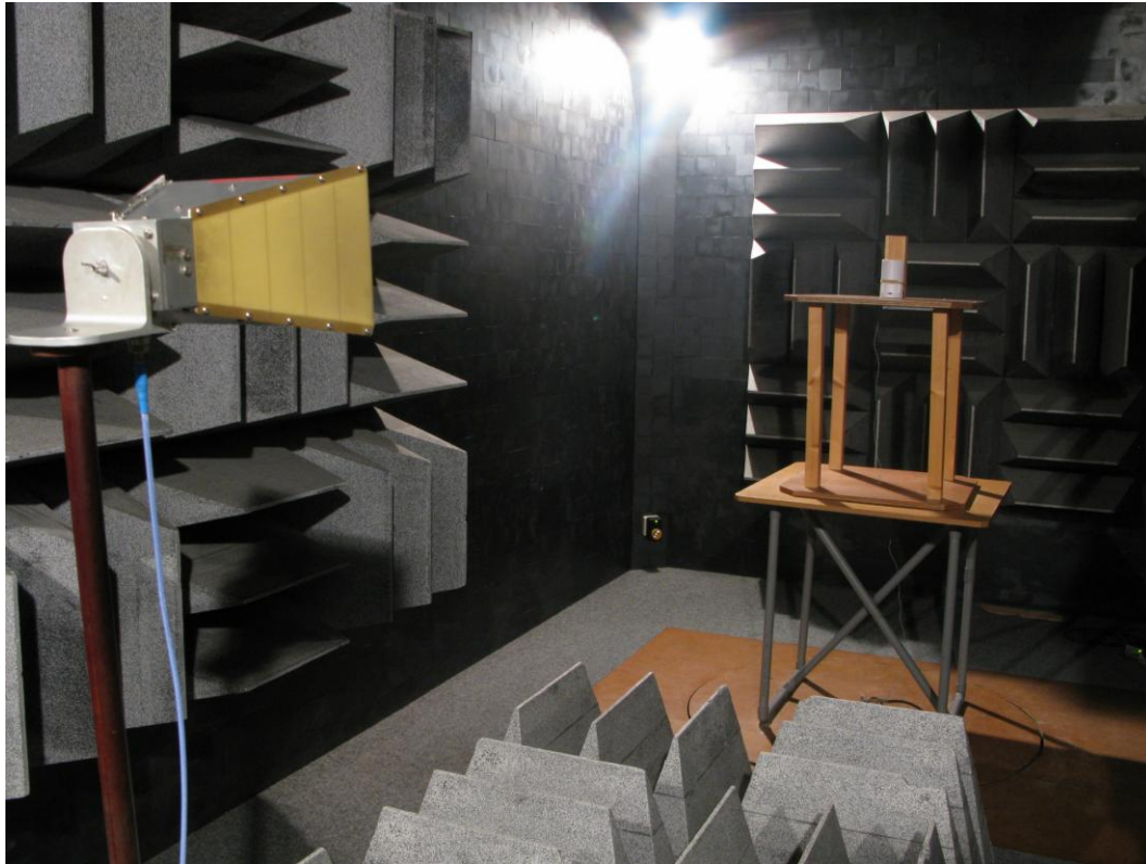
Photograph 2: Test setup radiated emissions (> 1000 MHz), 3m distance
