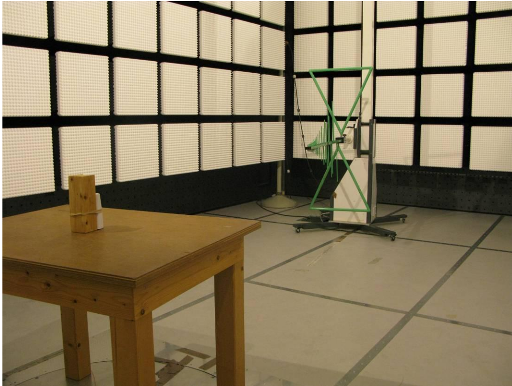
Photograph 1: Test setup radiated emissions (< 1000 MHz)
