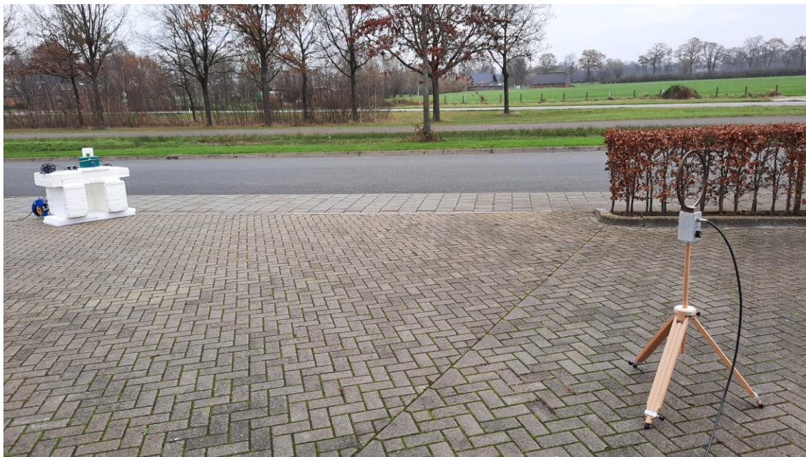
Setup EUT @10m (X-orientation shown)
