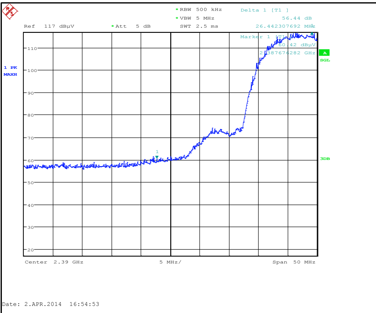
Plot 4-1: In Band Emissions - Channel 1 (2412 MHz); 802.11b (11 Mbps)
