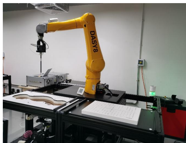
Picture D.6 Specific Absorption Rate Test Layout
