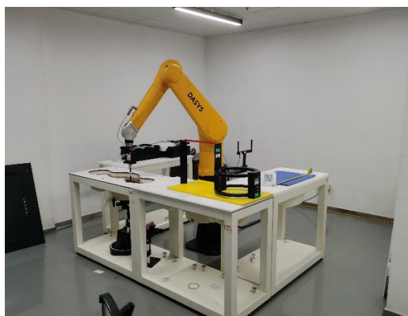
Picture D.6 Specific Absorption Rate Test Layout
