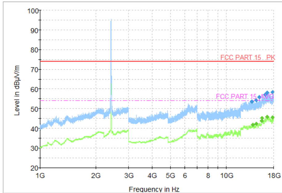
Fig.34 Radiated Spurious Emission (802.11b, CH1, 1GHz-18GHz)
