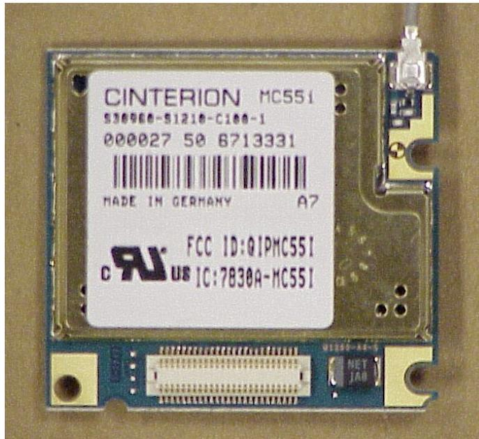
**THE MODULE AND ITS ANTENNA ARE MOUNTED ON A DAUGHTER BOARD:**
