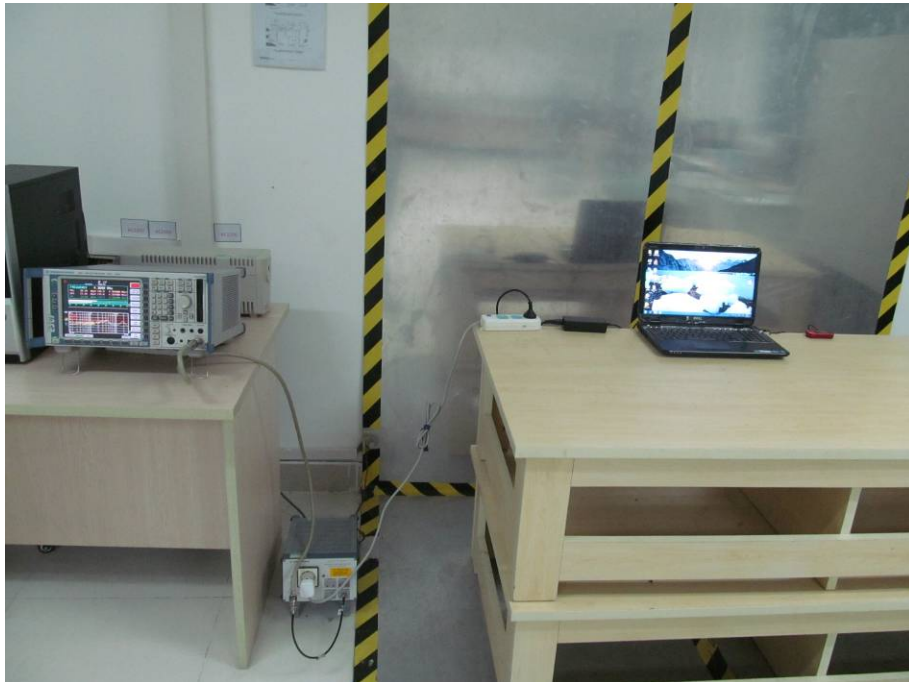
FCC LINE CONDUCTED EMISSION TEST SETUP
