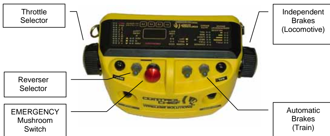
Figure 3-1: Lightweight OCU-BT Movement Controls
