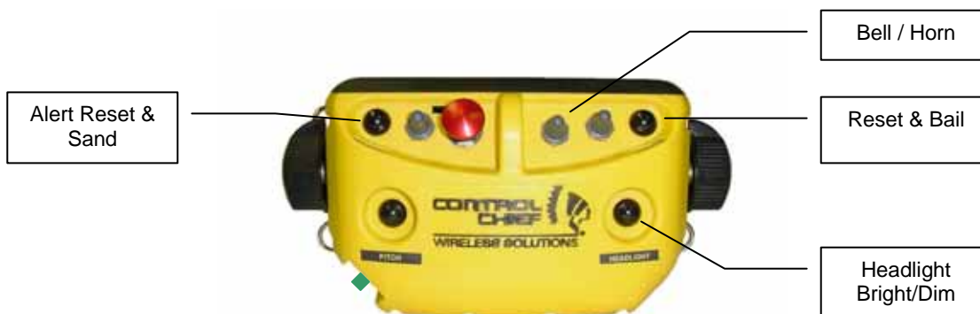
Figure 3-2: Lightweight OCU Misc. Locomotive Controls (Manual Brake/Throttle model shown)
