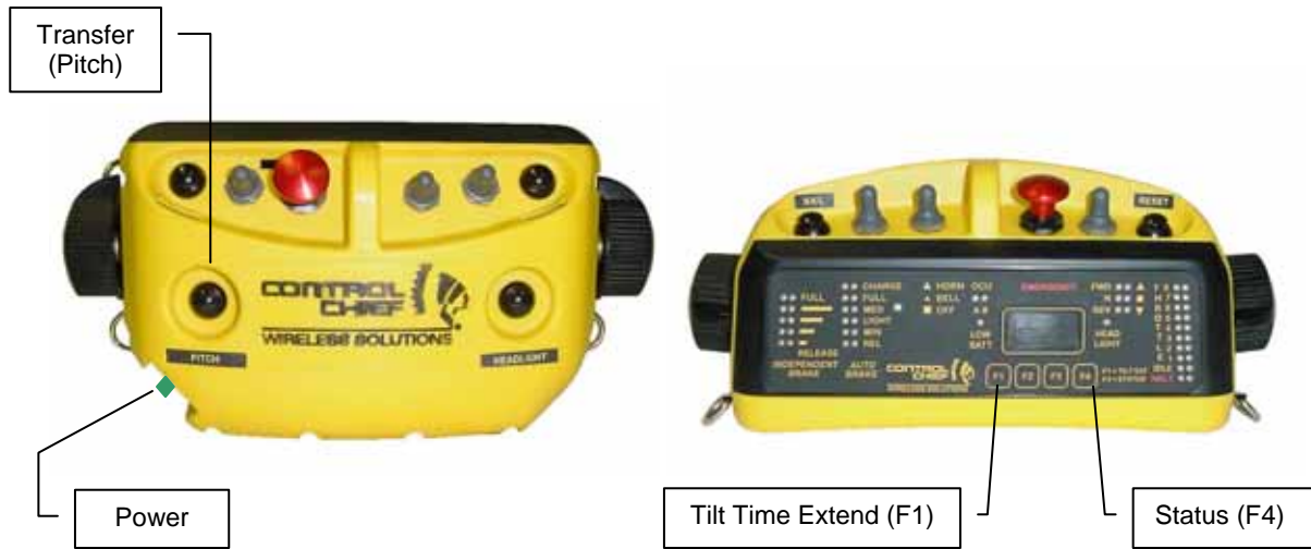
Figure 3-3: Lightweight OCU-BT Controls
