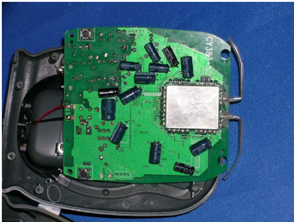
Base Main PCB solder side
