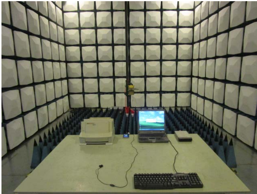
Radiated Emission –Front View (Above 1 GHz)
