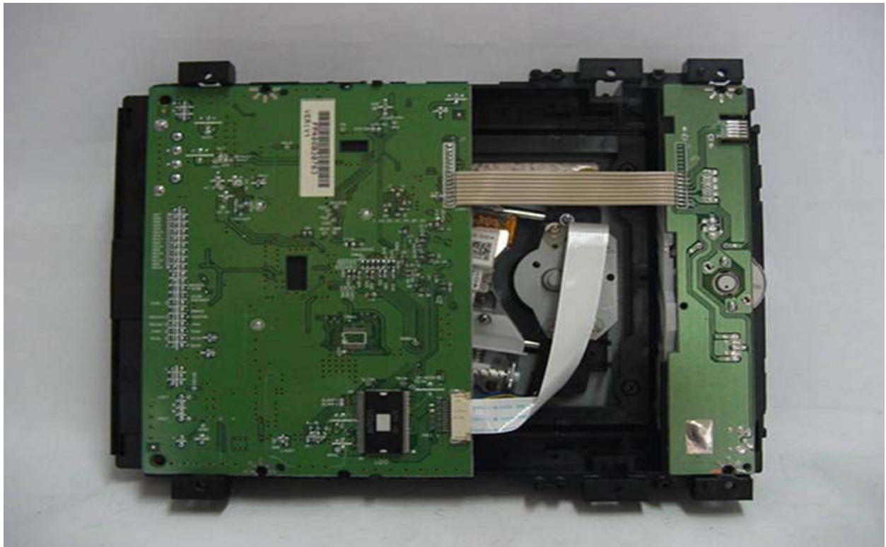
DVD Deck Bottom View (Removed Cover)
