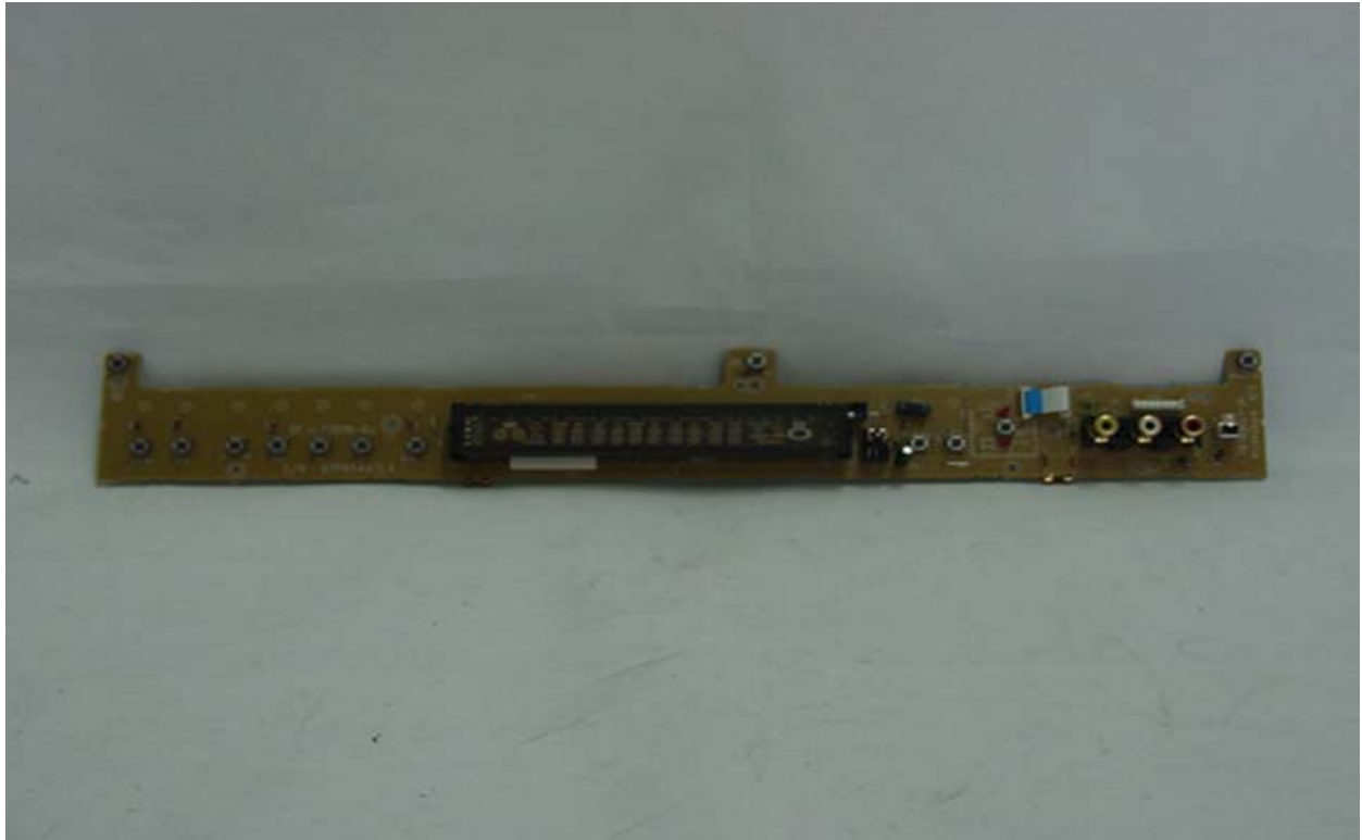
AUX front Input Panel & OSD Board PCB Parts View
