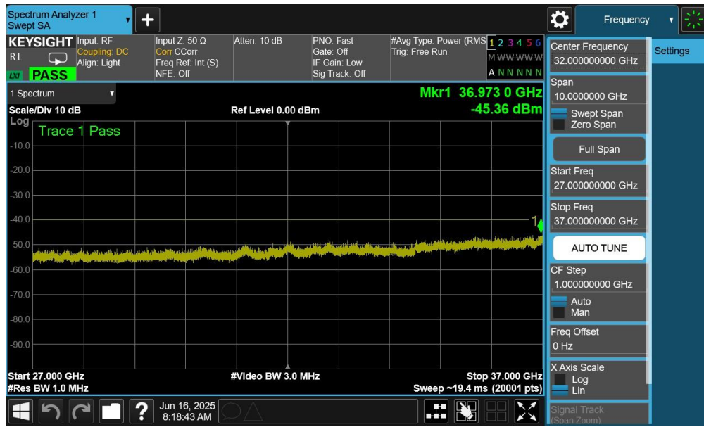
Plot 7-75. Conducted Spurious Plot (ULCA LB48 - 20+20MHz QPSK - High Channel - Ant6)
