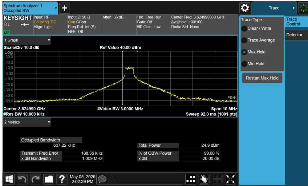
Plot 7-60. Occupied Bandwidth Plot (NR Band n48 - 40MHz 16-QAM - Full RB Configuration – SRS Ant4)
