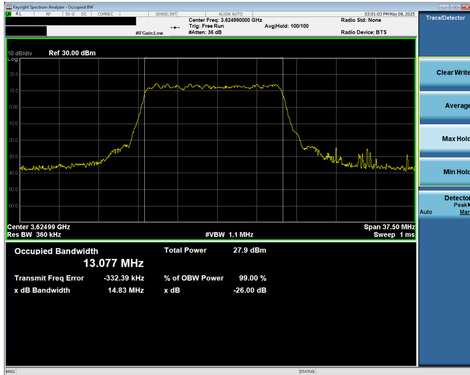
Plot 7-51. Occupied Bandwidth Plot (NR Band n48 - 15MHz 16-QAM - Full RB Configuration - Ant1)
