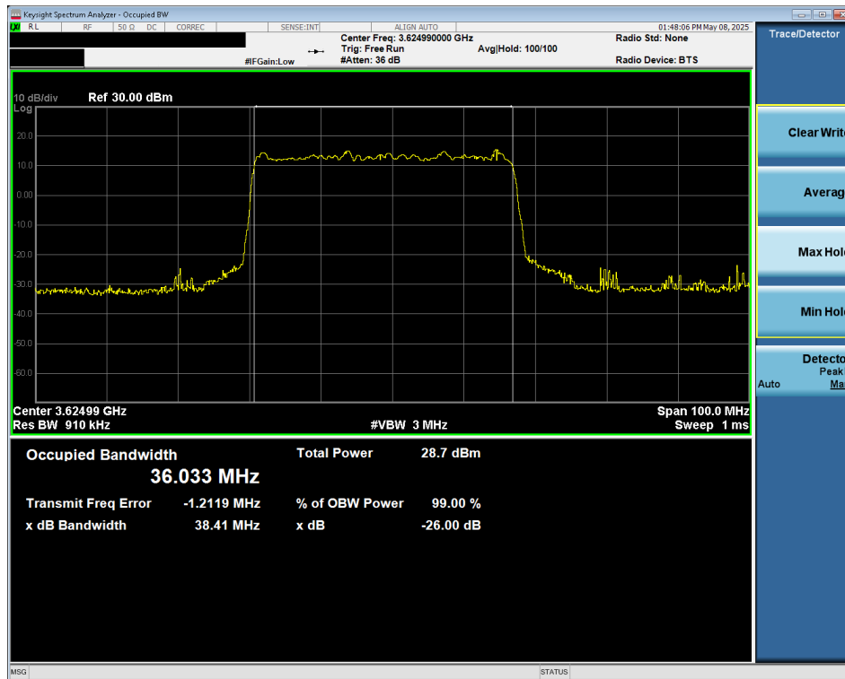
Plot 7-42. Occupied Bandwidth Plot (NR Band n48 - 40MHz 16-QAM - Full RB Configuration - Ant1)
