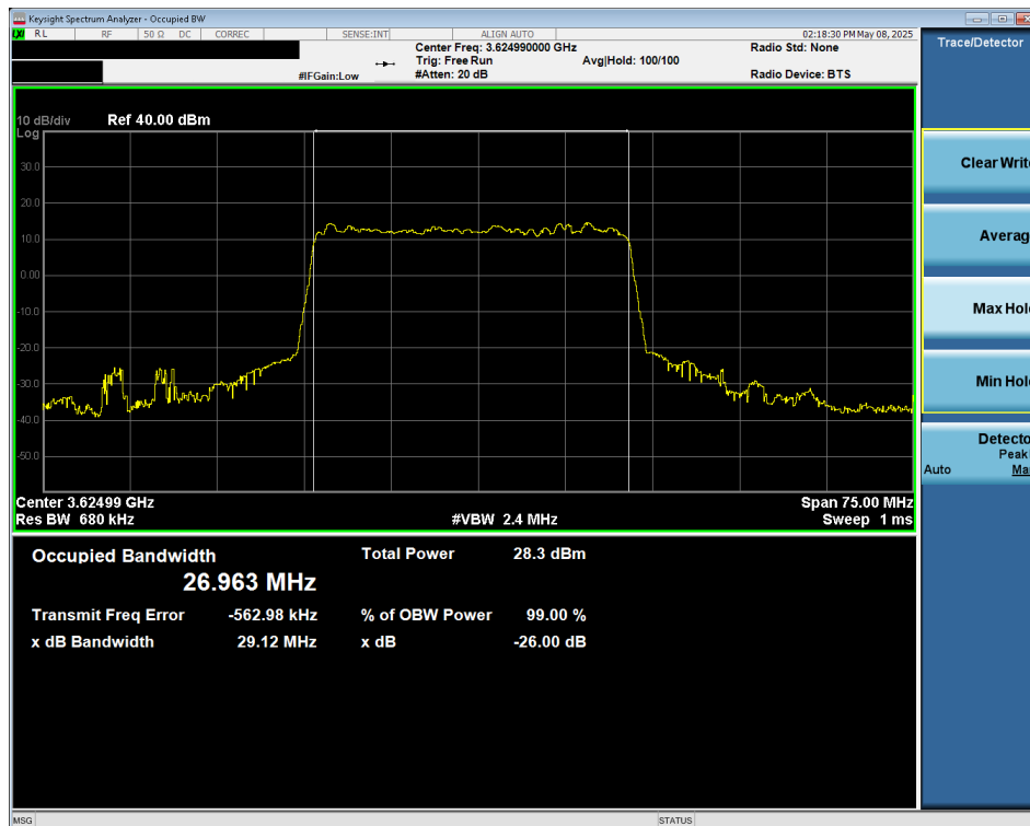
Plot 7-45. Occupied Bandwidth Plot (NR Band n48 - 30MHz 16-QAM - Full RB Configuration - Ant1)
