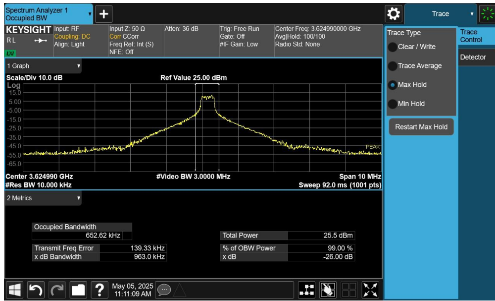
Plot 7-57. Occupied Bandwidth Plot (NR Band n48 - 40MHz 16-QAM - Full RB Configuration – SRS Ant3)
