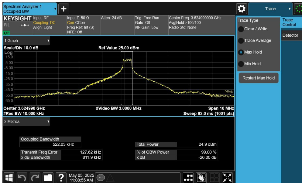
Plot 7-55. Occupied Bandwidth Plot (NR Band n48 - 40MHz \pi/2 BPSK - Full RB Configuration – SRS Ant3)
