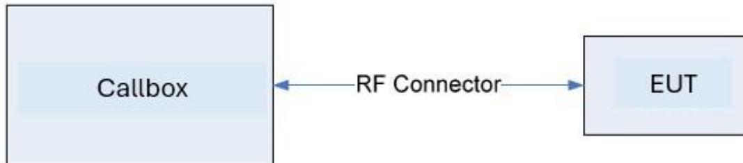
Figure 7-1. Test Instrument & Measurement Setup
