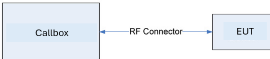
Figure 7-1. Test Instrument & Measurement Setup
