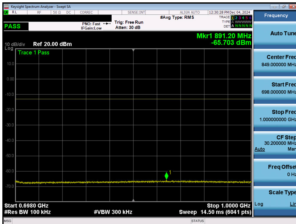
Plot 7-118. Conducted Spurious Plot (LTE Band 71 - 20MHz QPSK - 1 RB - Mid Channel - Ant 5)
