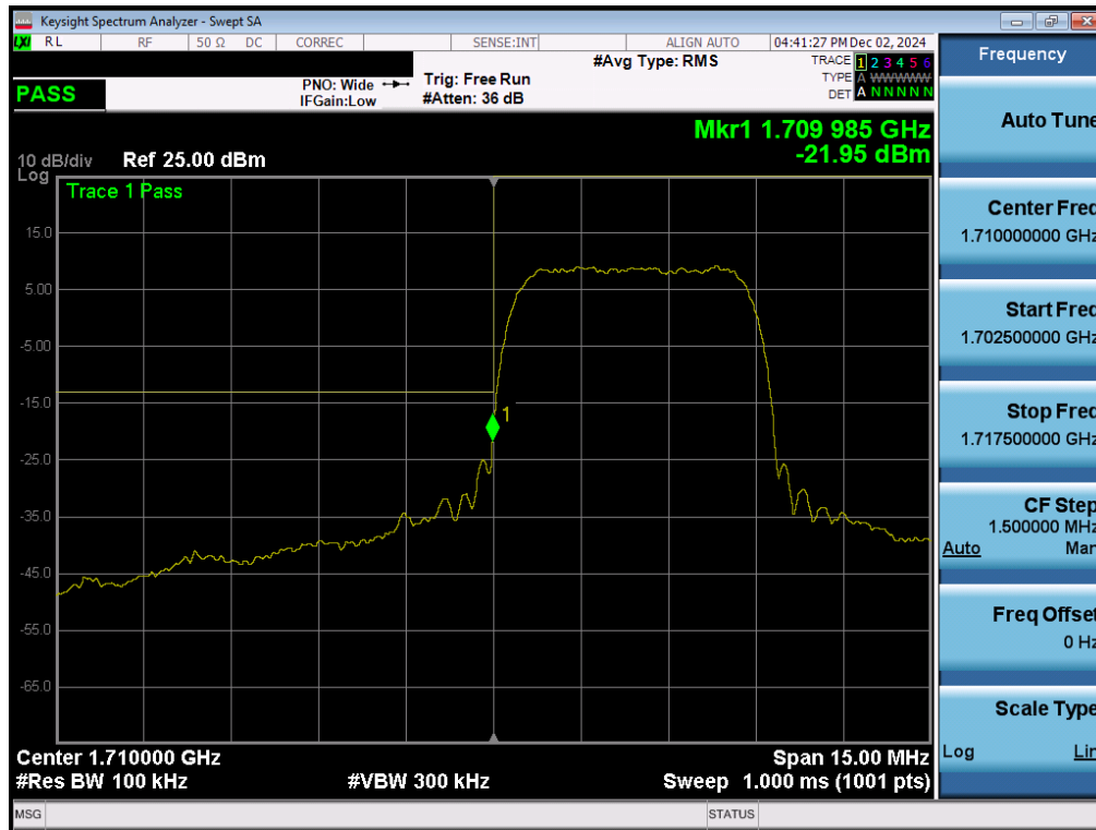
Plot 7-196. Lower Band Edge Plot (WCDMA AWS – Ch. 1312 – Ant 1)
