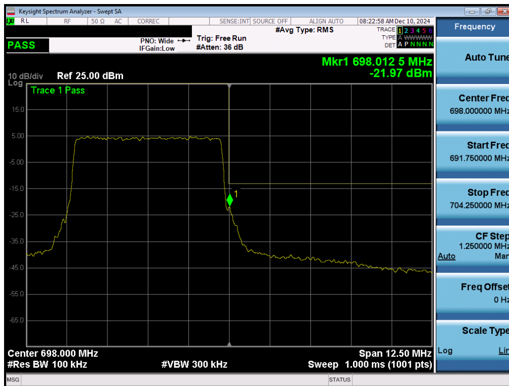
Plot 7-179. Upper Band Edge Plot (NR Band n71 – 5.0MHz - Full RB - Ant 5)
