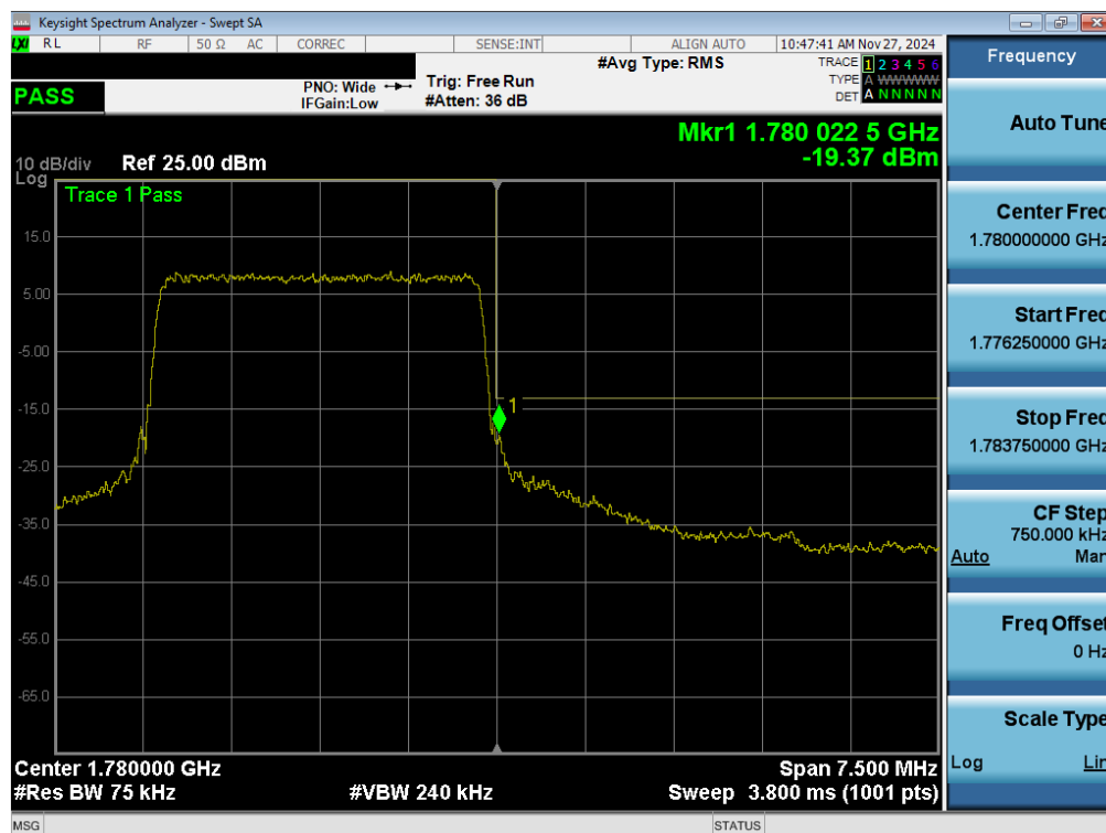
Plot 7-204. Upper Band Edge Plot (LTE Band 66 - 3MHz QPSK – Full RB - Ant 1)
