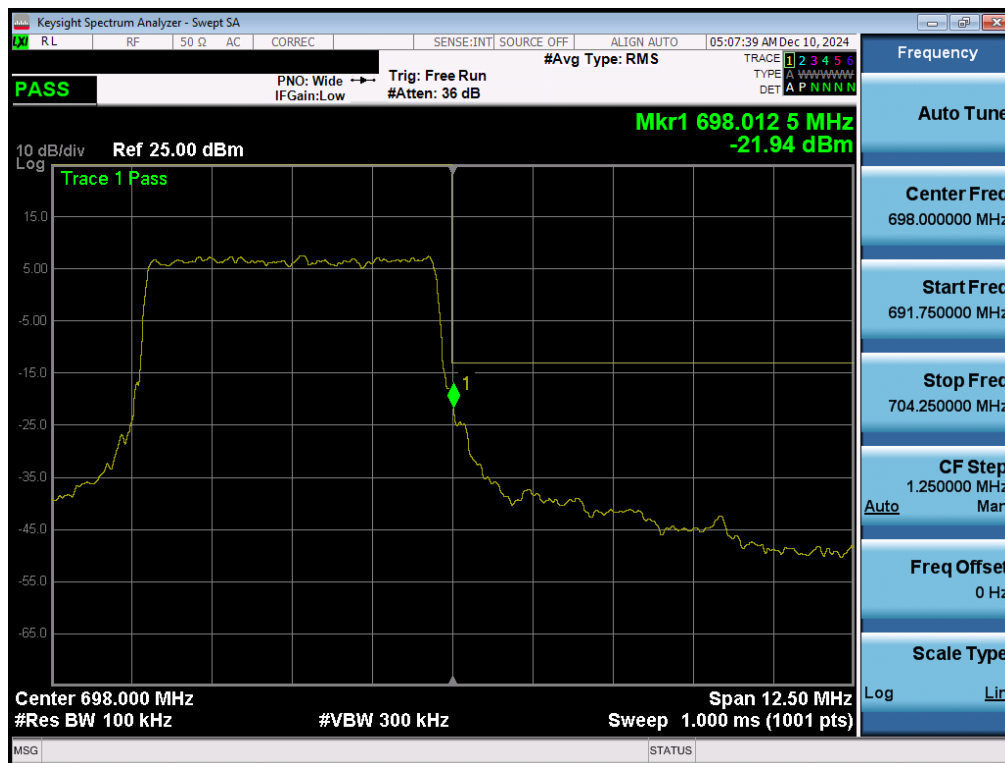
Plot 7-193. Upper Band Edge Plot (NR Band n71 – 5.0MHz - Full RB - Ant 2)
