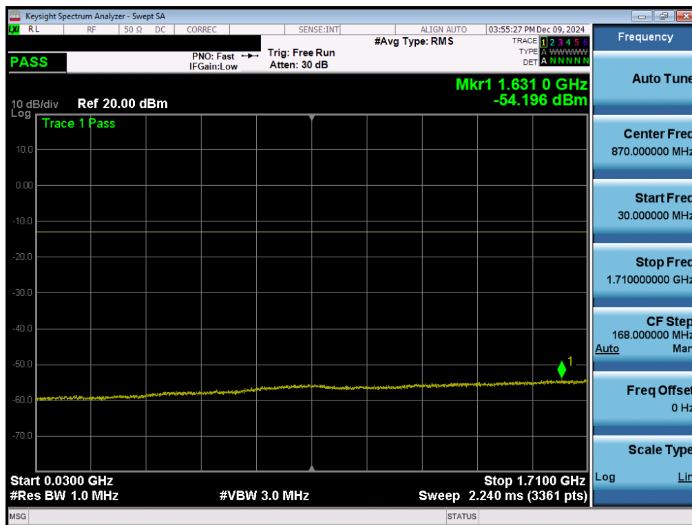
Plot 7-161. Conducted Spurious Plot (NR Band n66 - 40.0MHz - 1 RB - High Channel - Ant 1)
