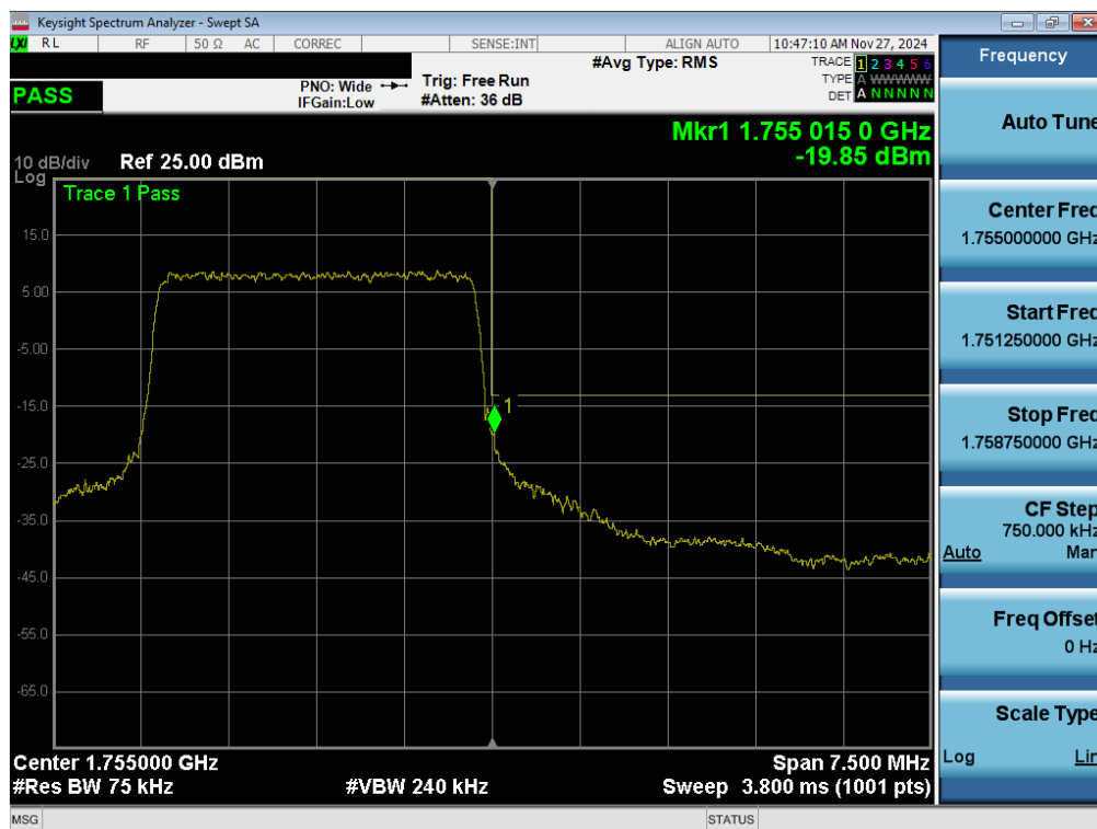
Plot 7-202. Upper Band Edge Plot (LTE Band 4 - 3MHz QPSK – Full RB - Ant 1)
