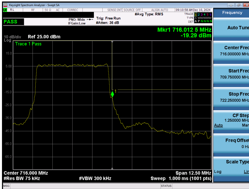
Plot 7-181. Upper Band Edge Plot (NR Band n12 – 5.0MHz - Full RB - Ant 5)
