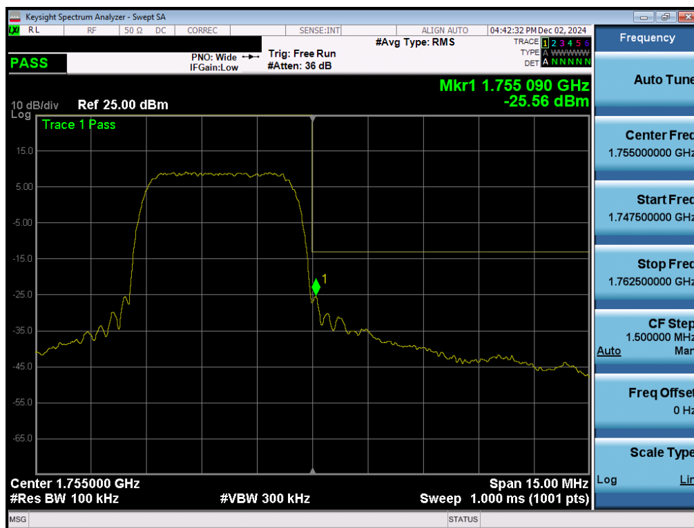
Plot 7-198. Upper Band Edge Plot (WCDMA AWS – Ch. 1513 – Ant 1)
