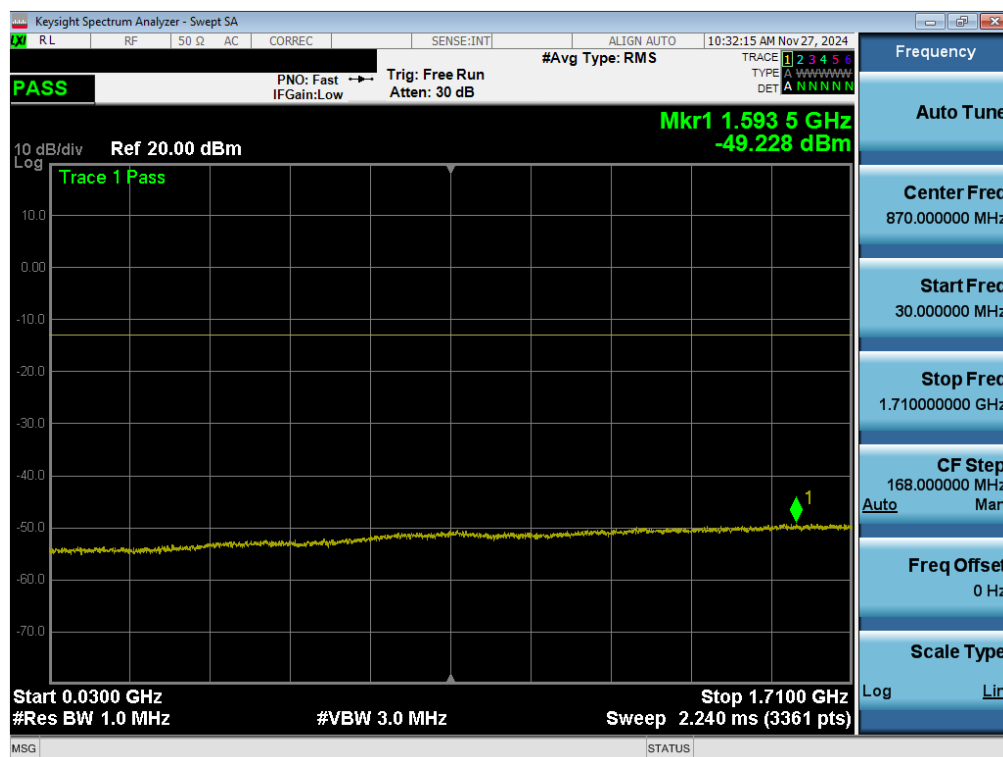
Plot 7-158. Conducted Spurious Plot (LTE Band 66/4 - 20MHz QPSK - 1 RB - Mid Channel – Ant 1)
