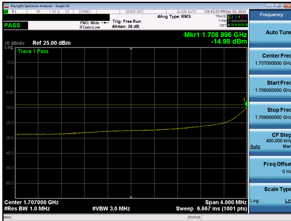
Plot 7-197. Lower Extended Band Edge Plot (WCDMA AWS – Ch. 1312 – Ant 1)
