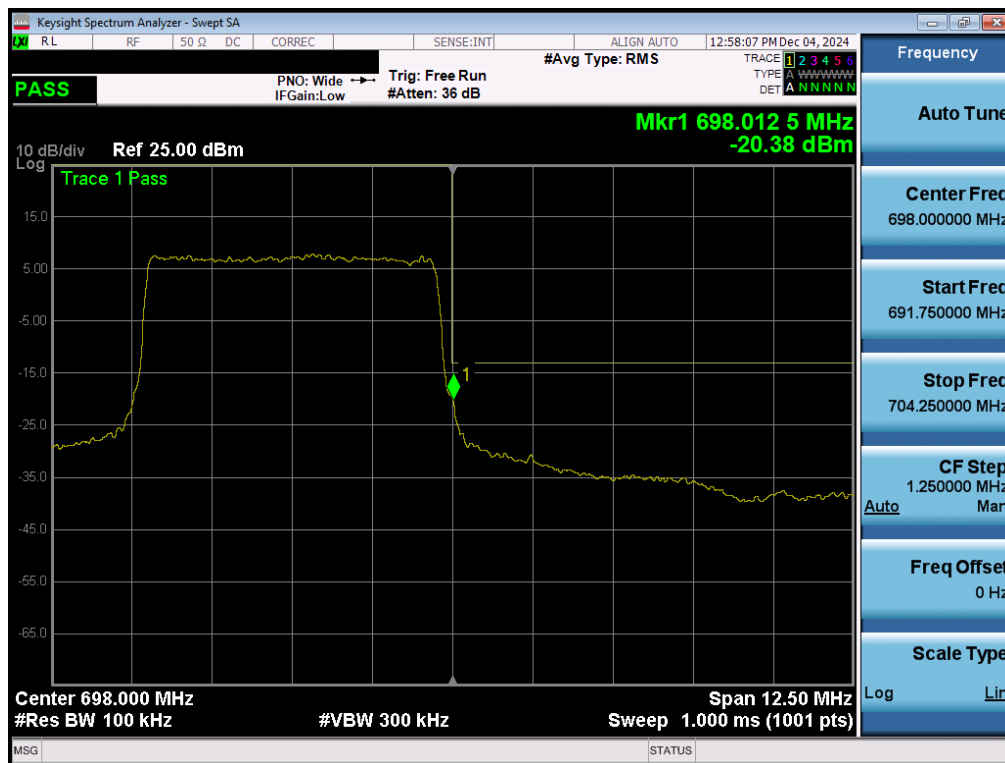
Plot 7-169. Upper Band Edge Plot (LTE Band 71 - 5MHz QPSK – Full RB - Ant 5)
