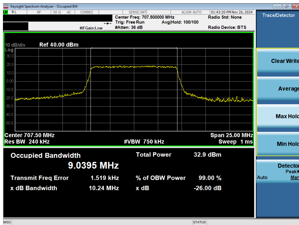
Plot 7-50. Occupied Bandwidth Plot (LTE Band 12 - 10MHz QPSK - Full RB – Ant 2)
