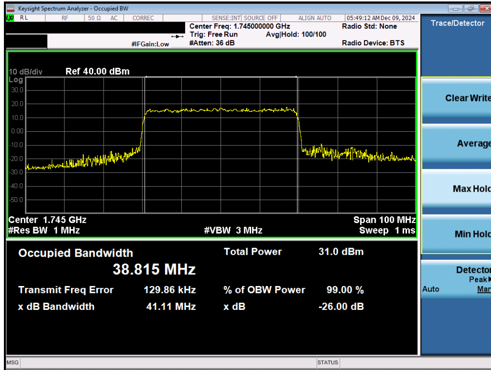
Plot 7-98. Occupied Bandwidth Plot (NR Band n66 - 40.0MHz CP-OFDM 16QAM - Full RB – Ant 1)
