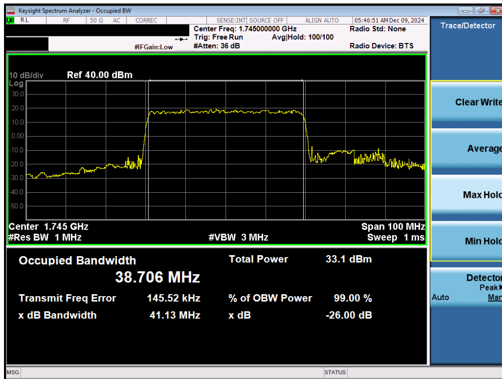
Plot 7-96. Occupied Bandwidth Plot (NR Band n66 - 40.0MHz DFT-s-OFDM BPSK - Full RB – Ant 1)
