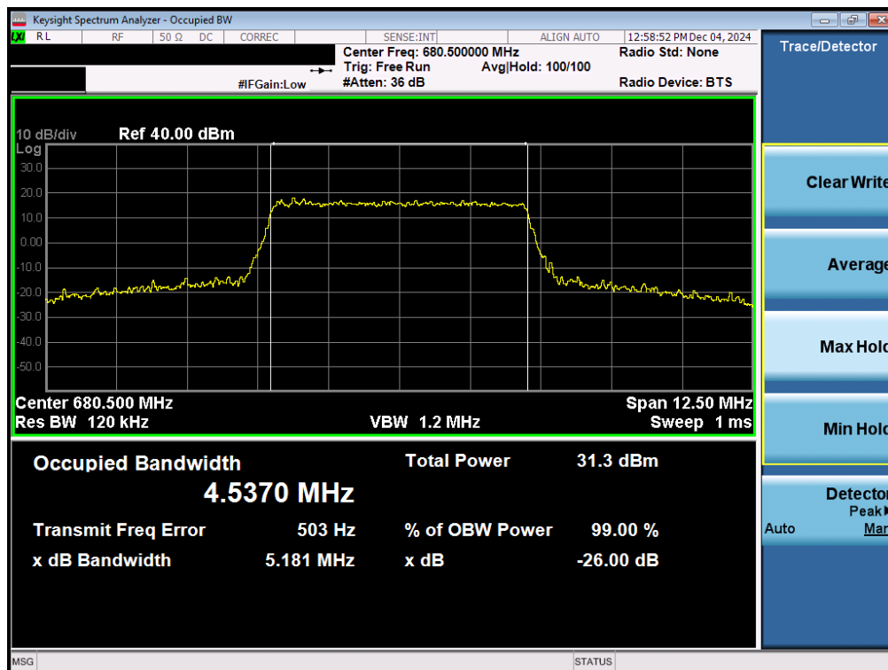
Plot 7-8. Occupied Bandwidth Plot (LTE Band 71 - 5MHz 16-QAM - Full RB – Ant 5)
