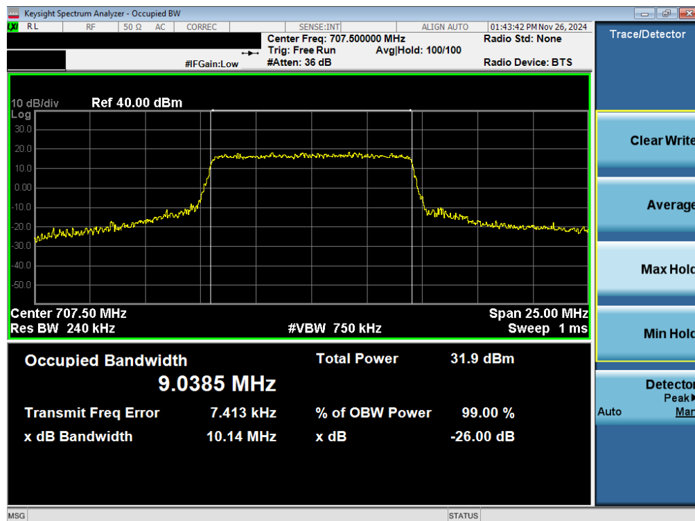
Plot 7-51. Occupied Bandwidth Plot (LTE Band 12 - 10MHz 16-QAM - Full RB – Ant 2)
