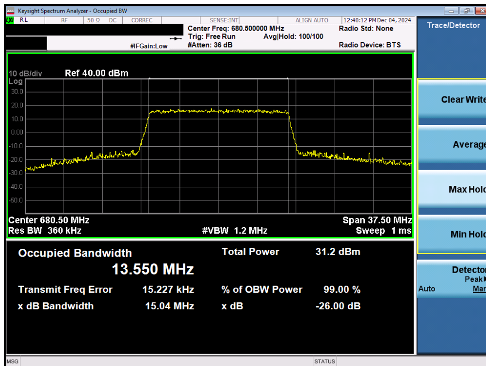
Plot 7-4. Occupied Bandwidth Plot (LTE Band 71 - 15MHz 16-QAM - Full RB – Ant 5)
