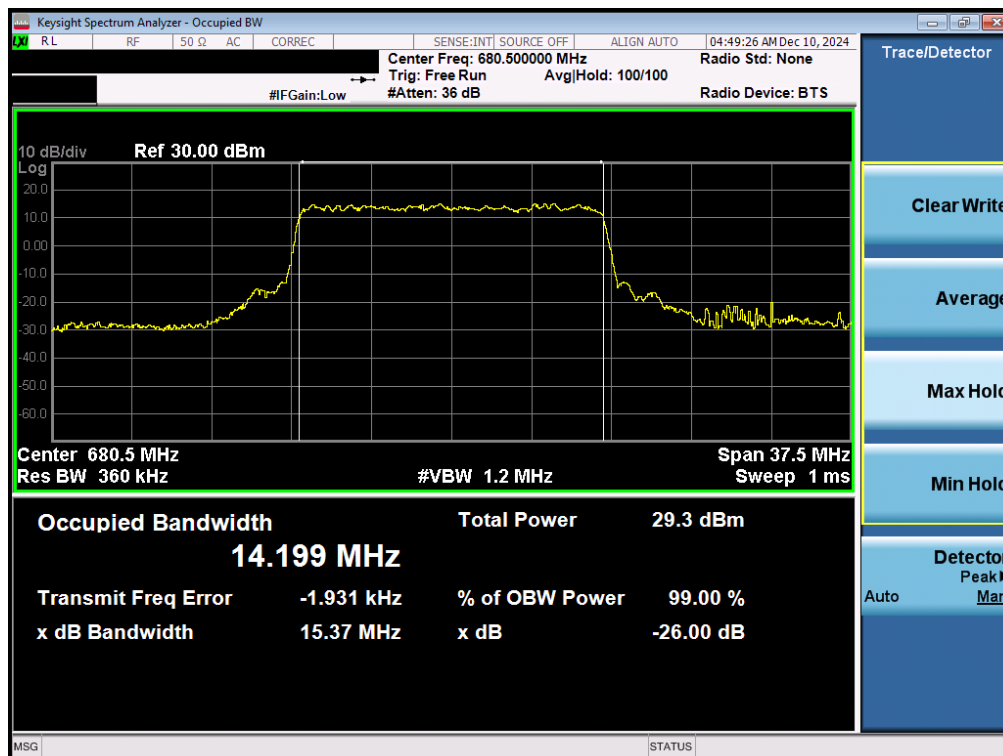
Plot 7-76. Occupied Bandwidth Plot (NR Band n71 - 15MHz CP-OFDM 16-QAM - Full RB – Ant 2)
