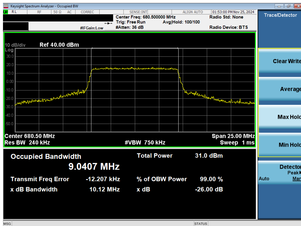
Plot 7-47. Occupied Bandwidth Plot (LTE Band 71 - 10MHz 16-QAM - Full RB – Ant 2)
