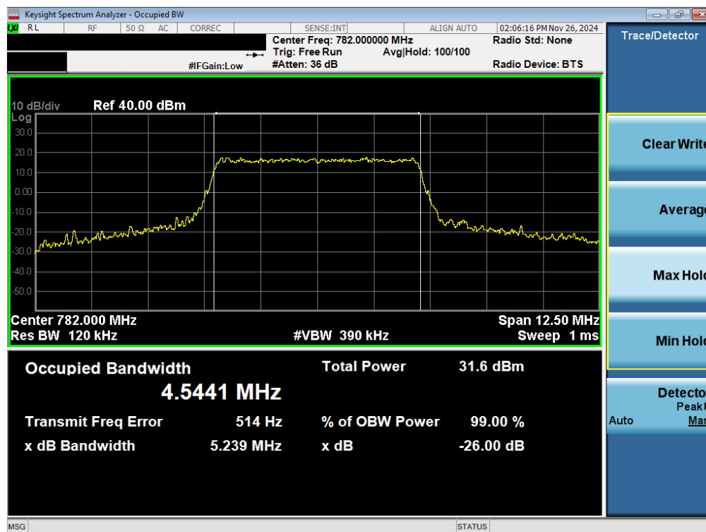
Plot 7-60. Occupied Bandwidth Plot (LTE Band 13 - 5MHz QPSK - Full RB – Ant 2)
