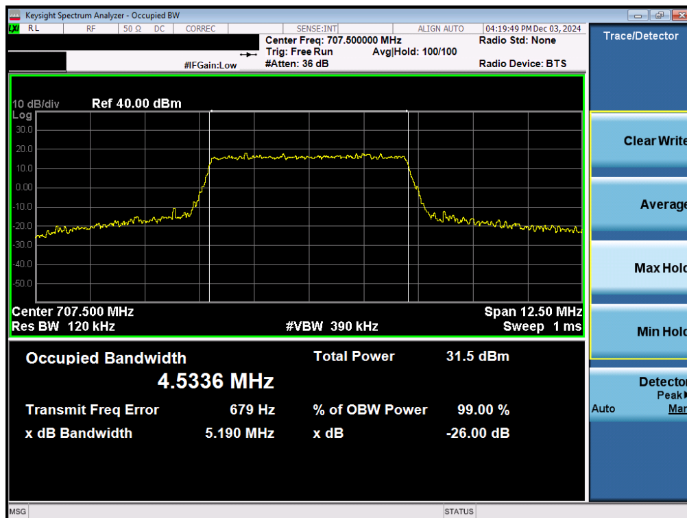
Plot 7-12. Occupied Bandwidth Plot (LTE Band 12- 5MHz 16-QAM - Full RB – Ant 5)
