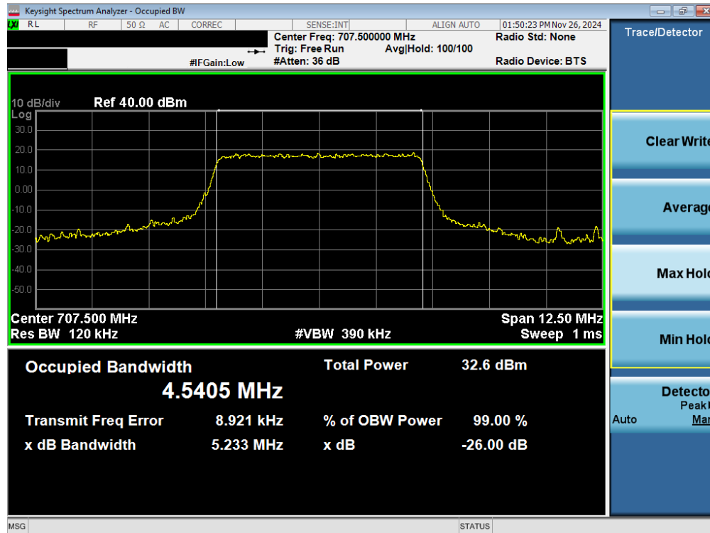
Plot 7-52. Occupied Bandwidth Plot (LTE Band 12 - 5MHz QPSK - Full RB – Ant 2)
