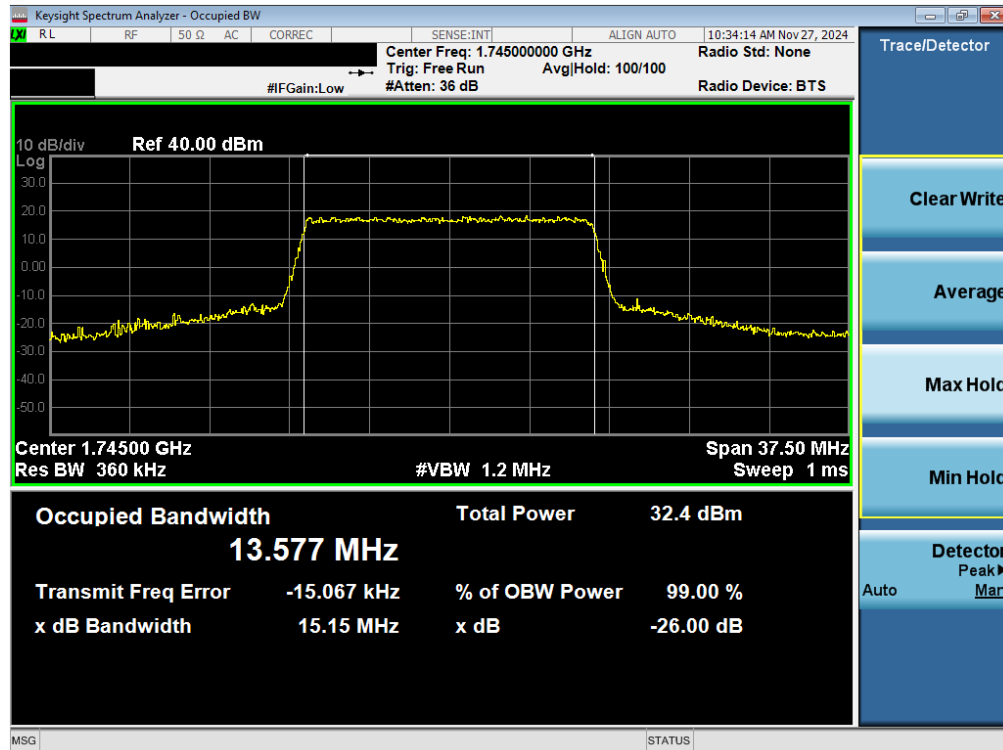
Plot 7-86. Occupied Bandwidth Plot (LTE Band 66/4 - 15MHz QPSK - Full RB - Ant 1)
