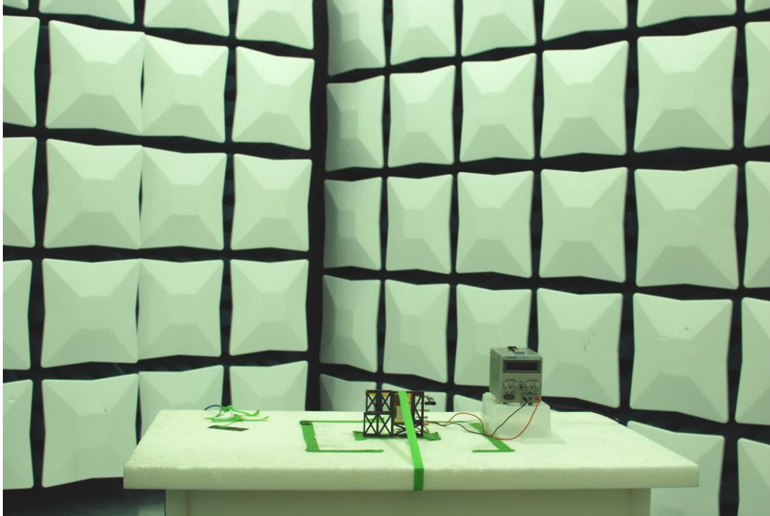
Figure 5. Test Setup – Y Position – 30MHz-1GHz
